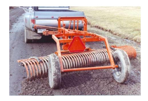
Hitch a Model HT to the back of a truck, tractor or any other motive power and perform dozens of road maintenance and landscaping tasks.
