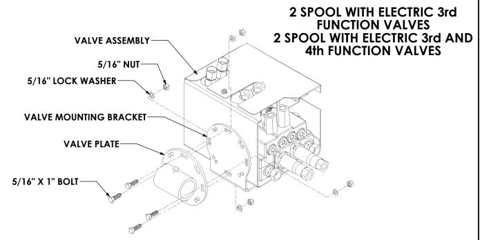
A) Attach the valve plate to the valve mounting bracket, as shown, using four 5/16" X 1" bolts, lock washers, and nuts provided.
