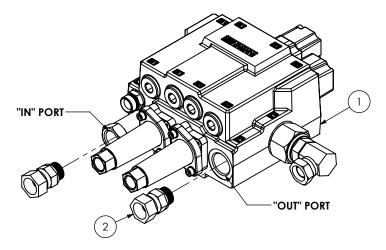
A) Attach two 3/4" X 1/2" swivels to the "IN" port and the "OUT" port of the valve, as shown.
