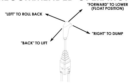
A) These are recommended operating positions for the joystick control. **NOTE:** When hooking up the loader you may need to move the hoses around until the loader operates the way you want it to.
