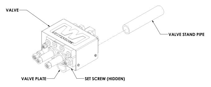
A) Attach the valve plate to the valve stand pipe, as shown, by sliding the pipe into the bushing on the bottom of the valve plate and tightening the set screw.
