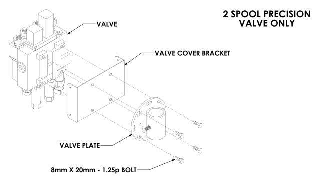
A) Attach the valve and the valve cover bracket to the valve plate, as shown, using four 8mm X 20mm - 1.25p bolts provided.
