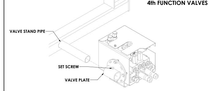
A) Attach the valve plate to the valve stand pipe, as shown, by sliding the pipe into the bushing on the bottom of the valve plate and tightening the set screw.
