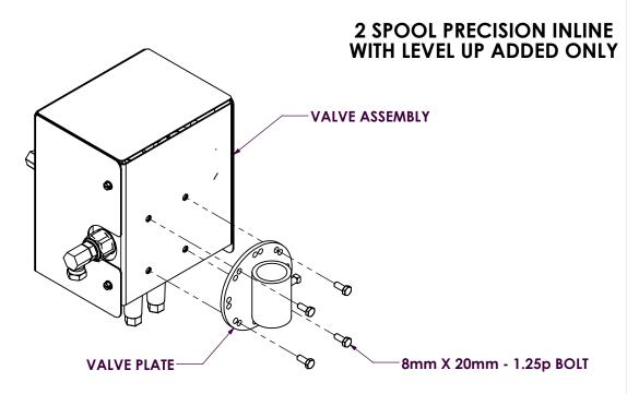
A) Attach the valve plate to the valve cover, as shown, using four 8mm X 20mm - 1.25p bolts provided. **NOTE:** The valve can be mounted in several different positions on the valve plate. Consider your hose lengths and joystick location when determining which holes to mount your valve.
