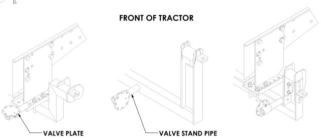
A) Mount your valve outside the cab in a location that will protect the valve from damage and will allow all the hoses and cables to be hooked up. This step may require some creativity on your part. Shown are a few examples of how the valve plate, and valve stand pipe can be mounted.
