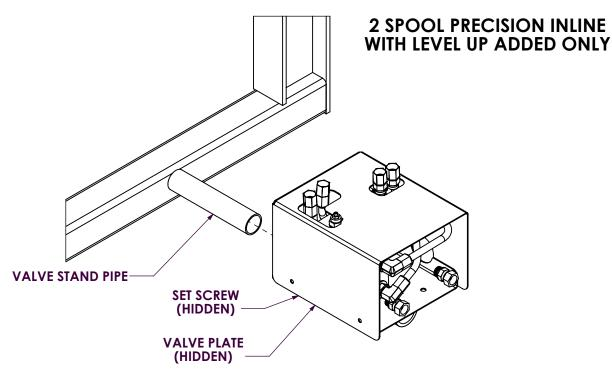
A) Attach the valve plate to the valve stand pipe, as shown, by sliding the pipe into the bushing on the bottom of the valve plate and tightening the set screw.
