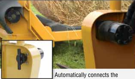
Automatically connects the feeding rotors with the hydraulic drive mounted on spear unit.
