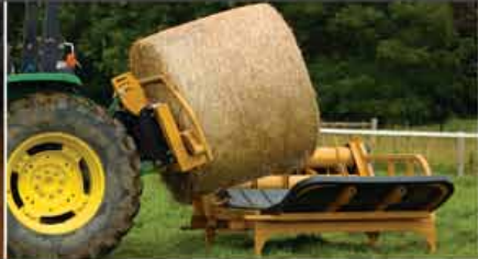
After loading the bale, the spear unit attached by sliding into the frame, creating a single carrying unit.
