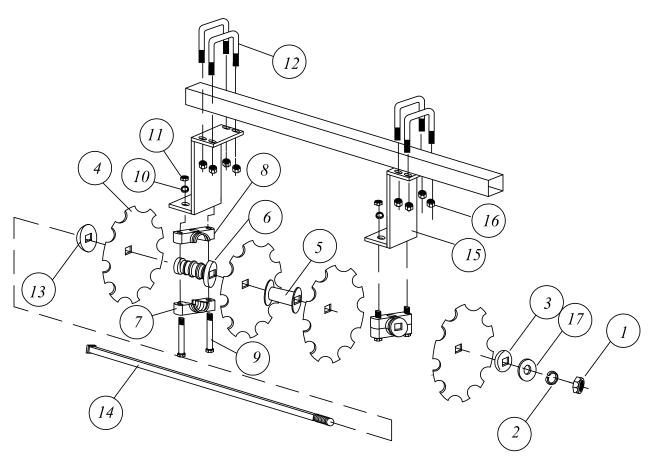
TGE 1" FRICTION BEARING GANG ASSEMBLY 1TGE71216F, 1TGE71218F 1TGE71616F, 1TGE71618F
