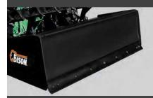
Soil displacement can be accomplished by forward and backward operations, due to the dual cutting edges available. Cutting edges are reversible and replaceable.
