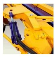
Retract the hitch pole cylinder in working position and replace the hitch pole safety pin.
