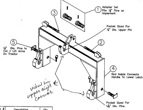
Item # Part # Description Qty 862530 **Bushing Kit** 2 2 862843 Handle (Only) 2 Grip for Handle 3 862844 2 4 862847 Rod (Handle to Latch) 2 Lower Mounting Pin 862846 LOADERS
