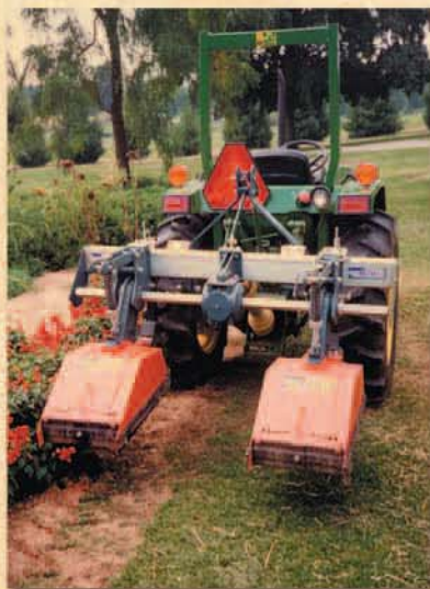
Model FP 66" frame with 2x12-16" tillage heads
