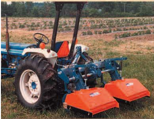
Model FL with 2 heads, clearing row middles during strawberry renovation
