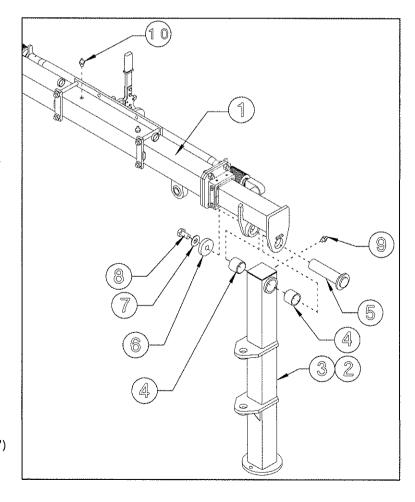
For correct assembly, the RH support 2 and the LH support 3 must lean in slightly towards the center of the machine. After assembly, they must have the measurements given. At this point, before moving on to step 5, keep in mind that the assembly is unstable and therefore it is recom mended that extreme caution be used.
