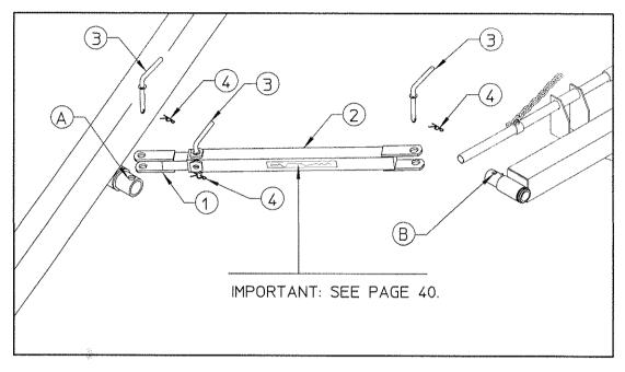
This is the assembly diagram for the MK10 and MK12. The row of holes on the arms is for when the rear axle is widened. Under no circumstances should the cylinders be operated while the transport arms are attached. The machine is now to be transported to the work site.
