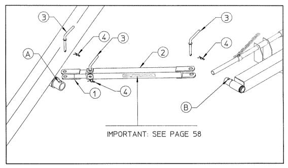
This is the assembly diagram for the MK10 and MK12. The row of holes on the arms is for when the rear axle is widened. Under no circumstances should the cylinders be operated while the transport arms are attached. The machine is now to be transported to the work site.
