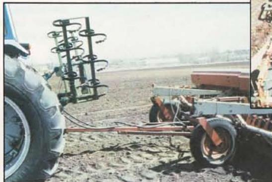
Folding WAC-A-TRAC improves turning radius. The WAC-A-TRAC will raise high enough to clear the implement hitch on most tractors.
