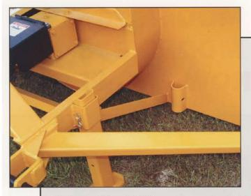
A post jack is standard equipment to help in hooking up and it positions the blower so water will drain from the fan when not in use. Skid shoes are standard equipment. They are adjustable for height. The skid shoe socket is welded to the housing at the factory.
