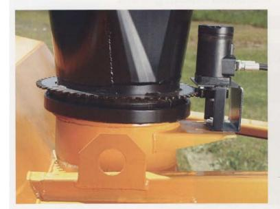
The hydraulic operated spout is built with a hydraulic motor and gear drive. The gear and motor mount are welded to the spout for ease of field installation. The spout has no stops and will turn continuously. There is no cable to wear out or break nor does the operator have to reverse the direction if he doesn't want to. The spout is rounded for smoothness of operation. The deflector back is also rounded and is adjustable by clamping with a tail nut.
