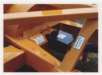
The Lorenz blowers are constructed of heavy gauge steel. All four corners are braced to the three point with heavy pipe.
