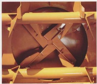
The four fan blades and cutting edge are replaceable.
