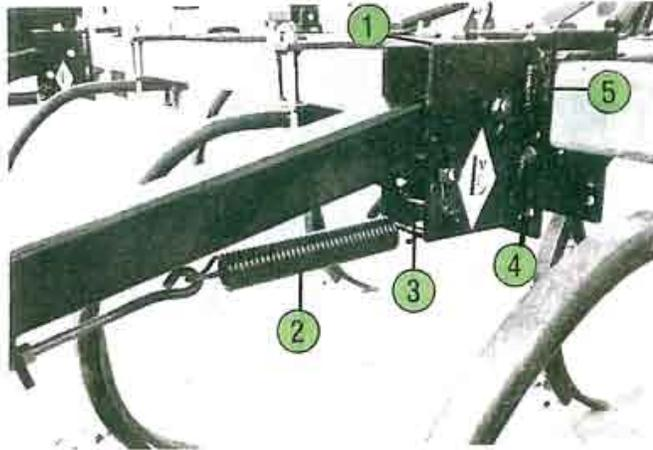
**1** HEAVY DUTY ARM MOUNTING BRACKET INSURES STURDY MOUNTING TO CULTIVATOR OR CHISEL PLOW.
