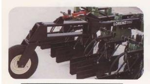
Lift Assist Wheel Kit Assy. - Optional Open Top Crop Shields - Optional Anhydrous Tank Pull Hitch -Optional (Not Pictured)
