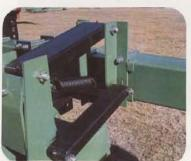
Triple Parallel Linkage Arms Locking Tabs - Gang to Beam Optional Down Pressure Spring
