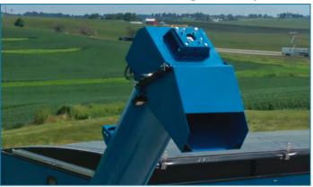
Simple tip spout grain control using tractor SCV
