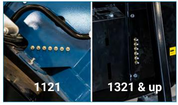
Centralized grease bank enables swift and easy lubrication
