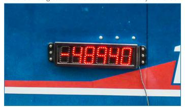
Optional remote scale readout for viewing by combine operator
