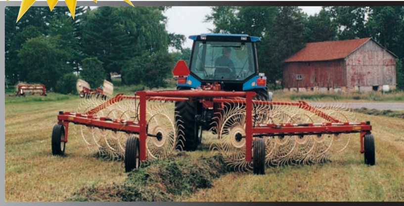
The high open, adjustable rear frame allows for the heaviest crop to pass through. Windrow width adjustment is done with a hand crank.
