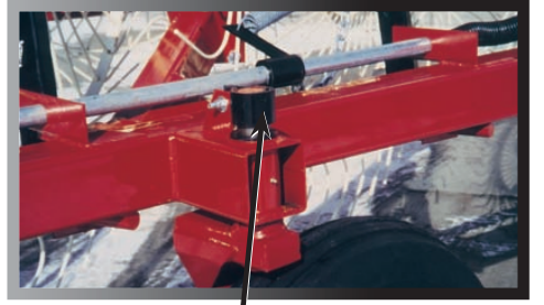
An adjustable brake band on top of the front spindle keeps the front gauge wheels from spinning in rough conditions.
