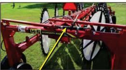
A **Ratchet Jack** is Standard for making Windrow Width Adjustments. The optional Hydraulic Cylinder w/Hoses requires a 3rd Hydraulic Tractor Remote.
