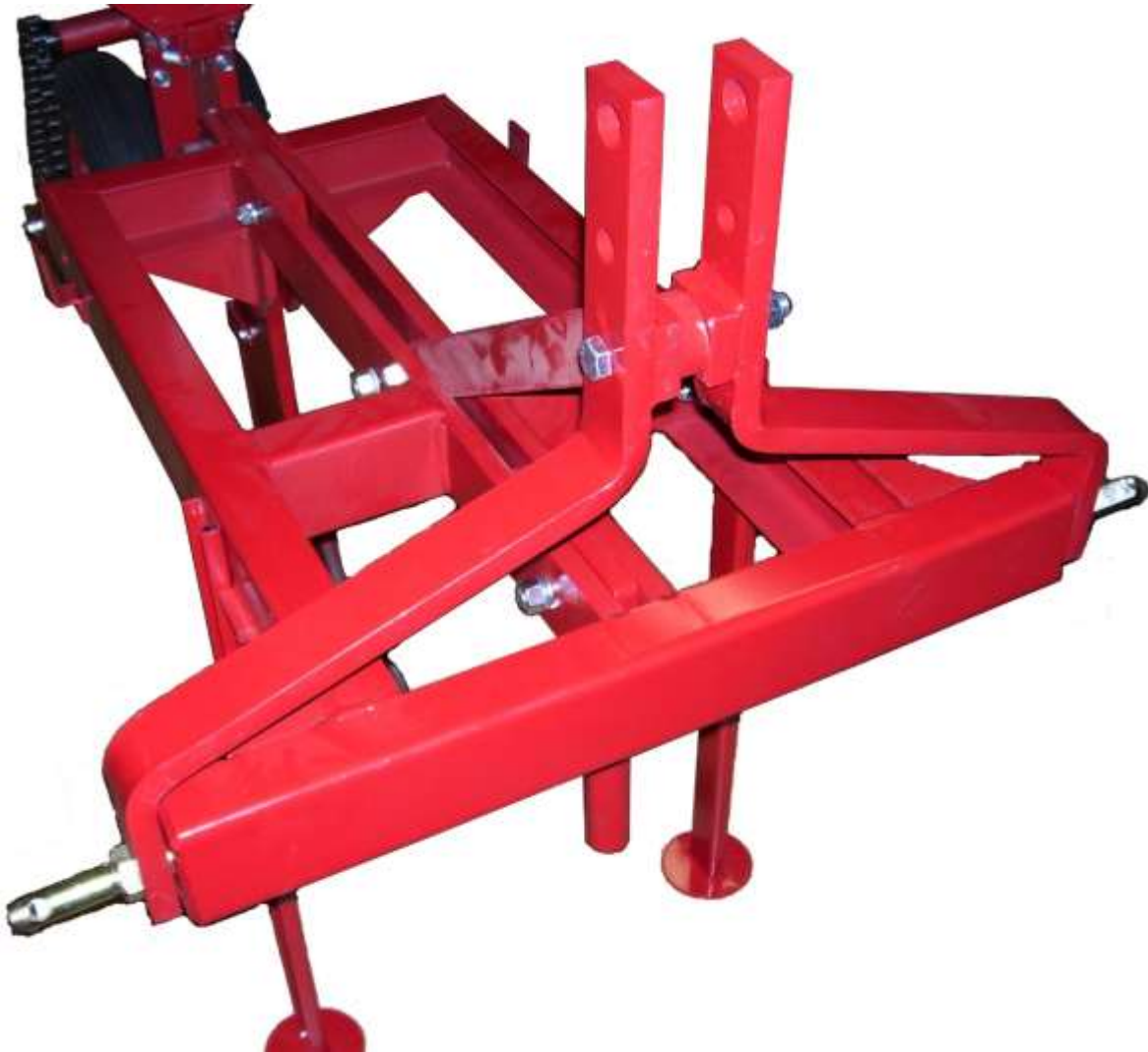
Figure 4: Lift Arm Tripod as Installed
