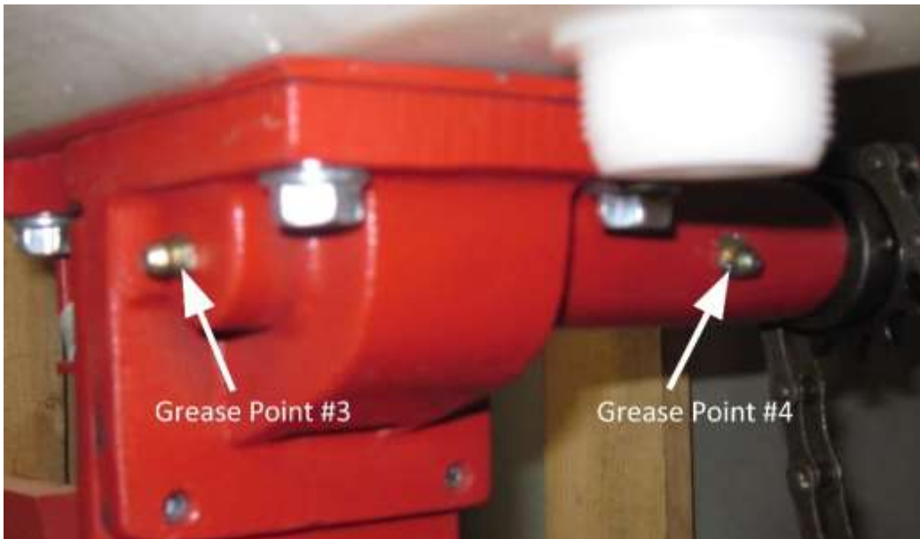
Figure 12: Seeder Casting Grease Points
