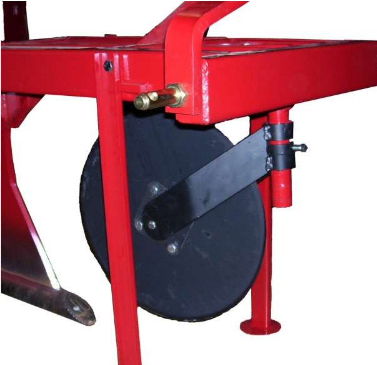
Figure 5: Coulter Assembly as Installed
