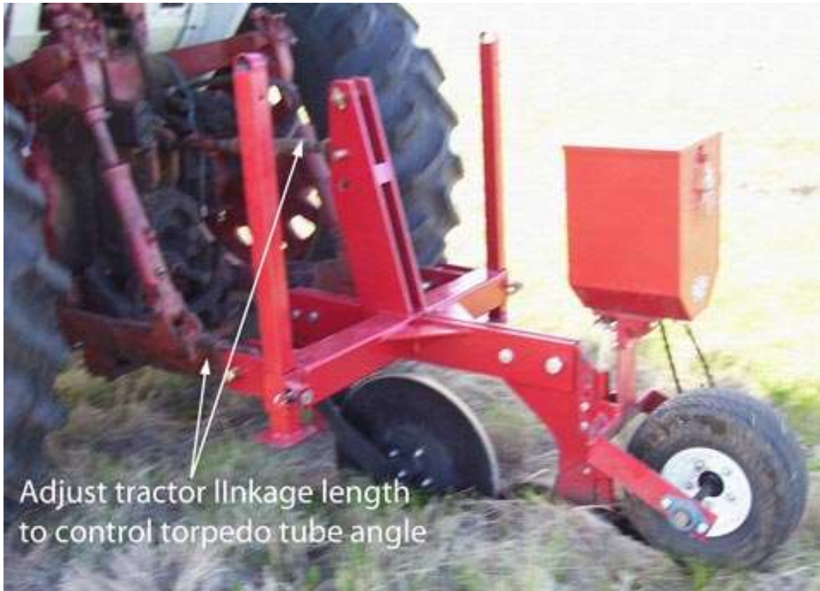
Figure 11: Adjustment of tractor link to control torpedo tube angle
