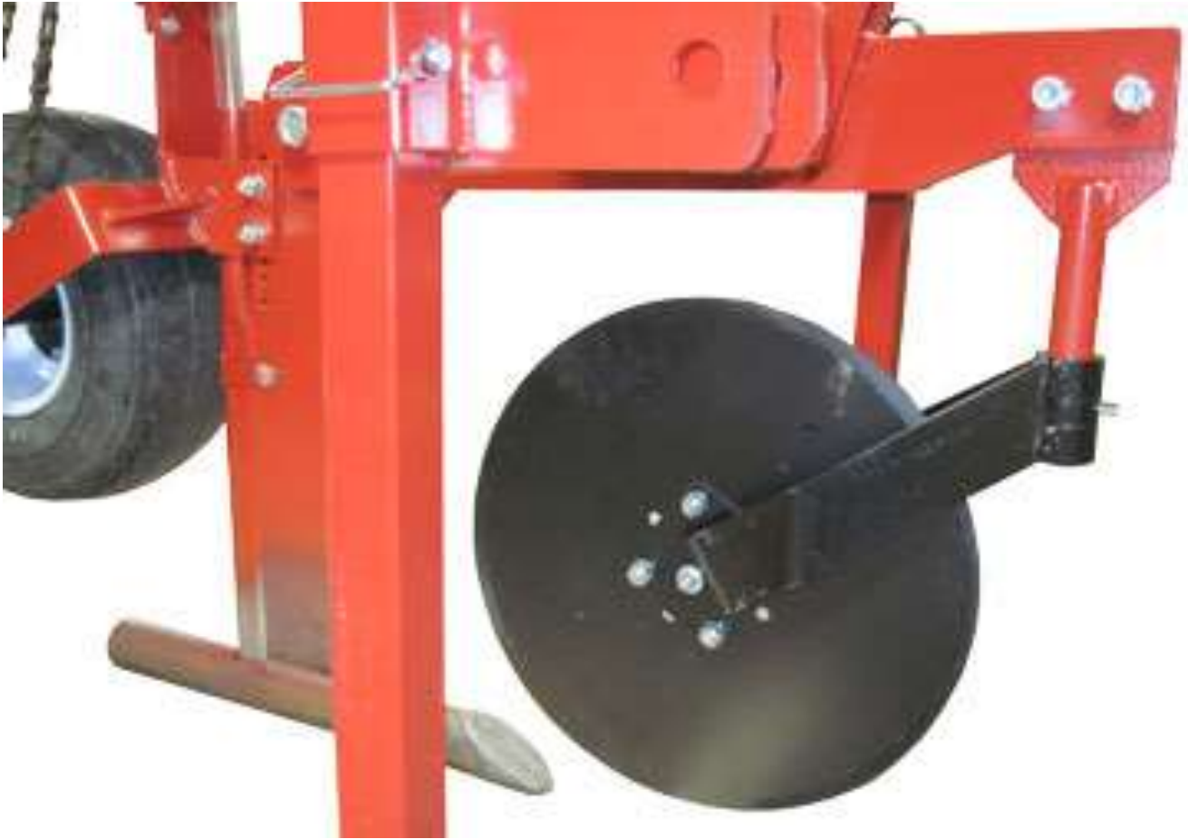
Figure 5: Coulters Assembly as Installed
