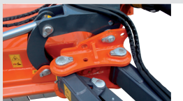
Rotation joint on self lubricating bushing.
