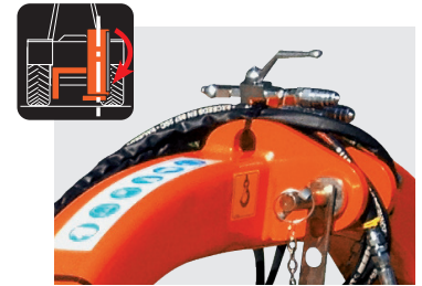
Hydraulic block tap for transport with manual activation (no chains or holders).
