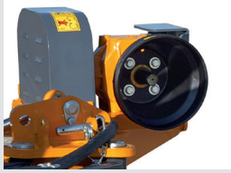
Gearbox external to the drive housing.
