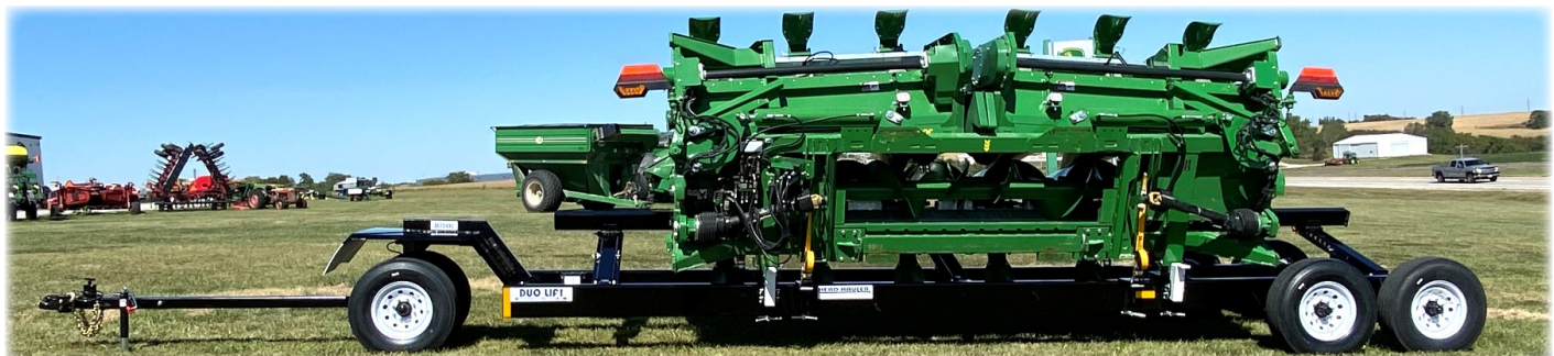
MODEL SHOWN: DLT24XL - IDEAL FOR CARRYING FOLDING CORNHEADS IN FOLDED POSITION FOR TRANSPORT.
