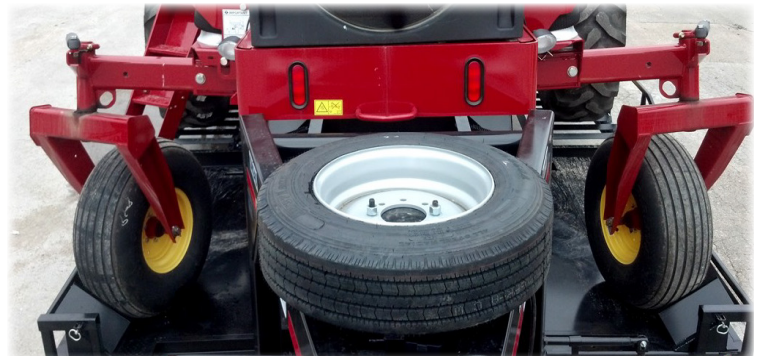
FOLDING CASTER WHEEL ROTATION AND SUPPORT PLATFORMS WITH ADJUSTABLE POSITION TIRE ANGLING GUIDE STOPS
