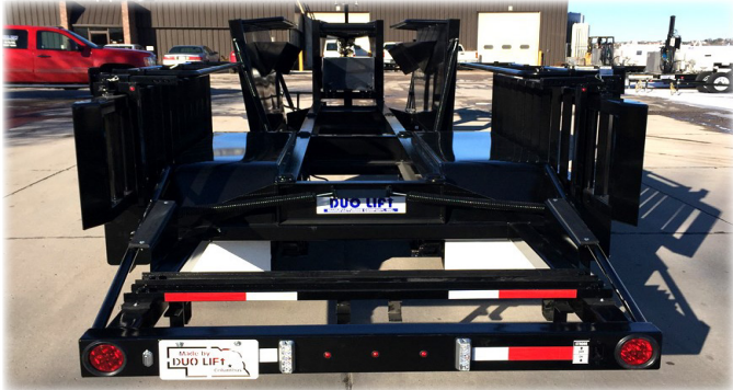
FOLDED TRANSPORT POSITION USING DUAL SPRING LIFT ASSIST FOR FOLDING ALL PLATFORMS. OPTIONAL 801158 STROBE LIGHT PACKAGE
