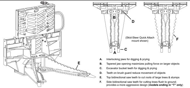
34" maximum jaw opening; maximum cylinder force of 21000 lbs.; synchronized interlocking jaws with excavator bucket teeth for digging, prying, and sawing; brush guard; and fully protected 138" hydraulic hoses with flat face ISO couplers.
