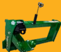
Offset Quick Attach Front-End Loader Mounts John Deere 200-500 Series (shown above), & Euro/Global
