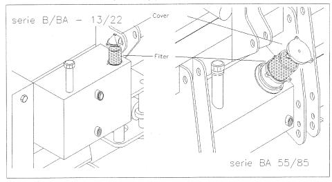
As for checking the filter it is necessary to remove the cover, unscrewing the screws, and pull it out from his seat (as shown in figure). If the filter is little dirty all it takes is cleaning it by blowing in compressed air (max 2 bar); if it had to be very dirty, instead, it is necessary to replace it. Use only a new filter and of the same type.
