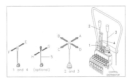
**NOTE:** moderate shifts of the levers allow to perform little and gradual movements. With levers at the limit stop it is allowed the highest speed of movement. Do not keep long the levers at the limit stop so as to avoid overheating the hydraulic oil.
