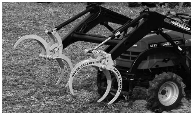
The teeth will open or close independently of each other based on the amount of hydraulic resistance
