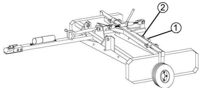
**IMPORTANT:** If you purchased a land plane with an electric actuator it is very important that you always properly lock the wheel carriage before transporting your land plane. Failure to do so will damage your actuator and void your warranty.
