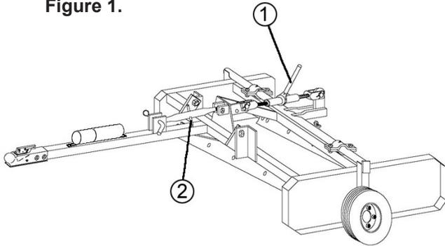
buckle (Figure 1, #1), lower your land plane about 1" off of the ground. Check and see if the front cutting blade is higher or lower than the rear cutting
