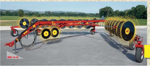
Inorder to adapt to extreme field conditions, hay rakes must be solid and sturdy. This is why the drawbar and the rake wings have been made using a large lattice framework of structural tubing to make their tough and fully reliable over time, however hard they are made to work. Despite their size, these machines are easy to handle and transport and very user-friendly.
