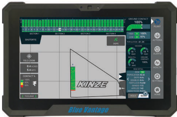
True Depth map showing target gauge wheel load percentage of ground contact
