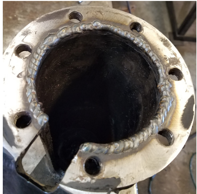
Fig. 3: Spot welds around flange circumference
