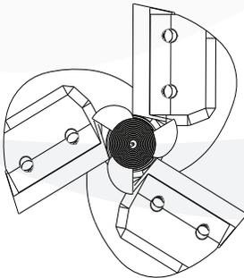
The stump auger planes away stumps without requiring large, specialized equipment. A threaded pilot digs into the stump and large cutting blades then shave the stump away. The large cutting blades are reversible for more cutting life. Complete stump removal is achieved by overlapping planning locations.
