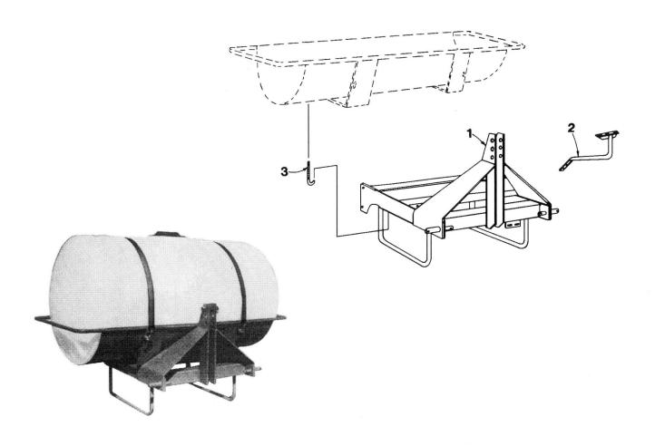
Note: Use (2) 1/2" x 1 1/4" Bolts To Mount The Saddle In Front and (2) 1/2" J-Bolts To Mount The Back Side Of The Saddle To The Frame.
