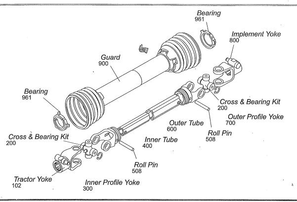
Each series has an exploded view for identification purposes. The drawing illustrates the components in the same sequence as an implement input driveline transmitting power from tractor to implement. Each component of the exploded view is identified by an eight-digit stock number to insure correct identification of each component.
