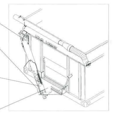
Minimum hydraulic requirements: 8 GPM @ 1200 P.S.I.
