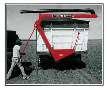
The unit is mounted completely on the exterior of the truck to allow for full tarping of the load.
