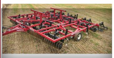
The Finalizer combines Cobra<sup>™</sup> disk blades with a patent-pending Talon<sup>™</sup> sweep to increase water movement and promote better root growth.
