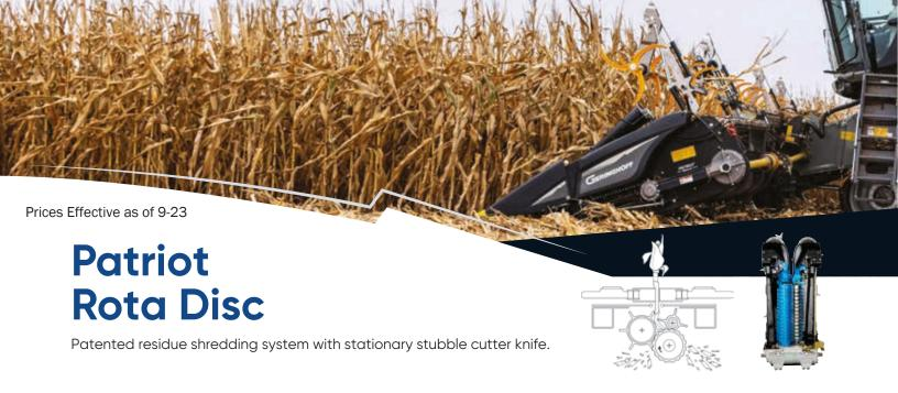
Using the chopping Rota Disc system, the wide angled gathering chains of the Patriot leaves a more open design of the entry area allowing for a gentle crop intake. This head has the flexibility to harvest single or twin rows in any condition.
