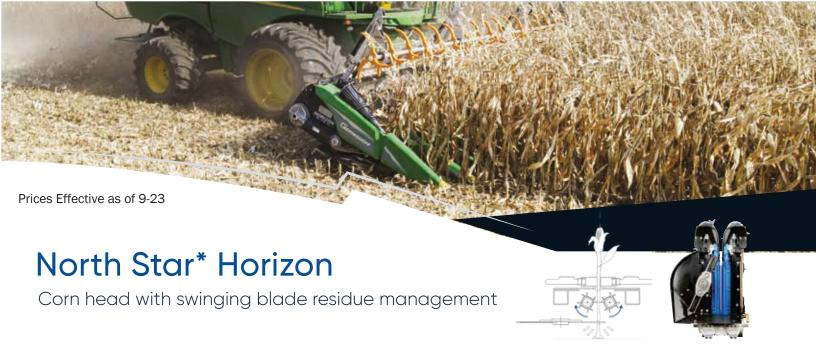
Dual knife roll head equipped with swinging blade chopper that can be disengaged, when desired. The swinging blade reduces the stalks to uniform lengths and spreads chaff evenly, which leads to optimum decomposition. This system is ideal for row spacing of 20"-40".
