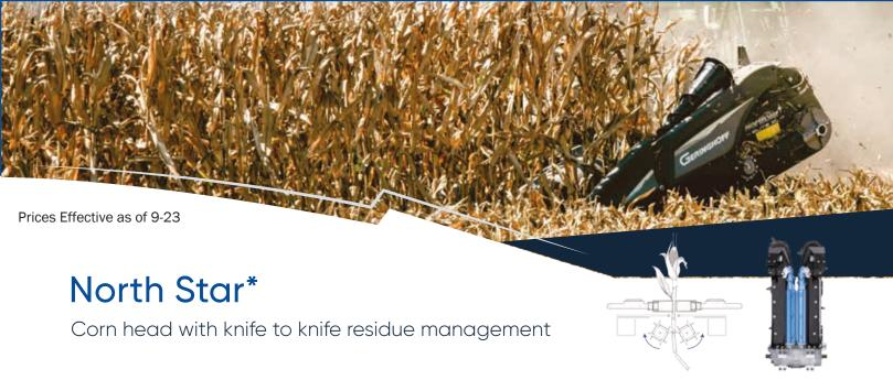
Two counter rotating snapping rolls with four knives each to provide maximum stalk cutting. This system is ideal for row spacing of 20"-40".
