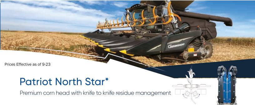
Using the well-know North Star\* system, the wide angled gathering chains of the Patriot leaves a more open design of the entry area allowing for a gentle crop intake. This head has the flexibility to harvest single or twin rows in any condition.
