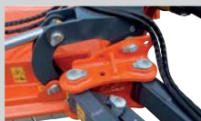
Rotation joint on self lubricating bushing.
