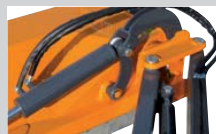
Rotation joint on self lubricating bushing.
