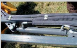
Hydraulic side shift cylinder fitted within the parallel arms for better protection during work
