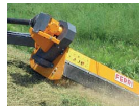
Gearbox unit outside the transmission cover
