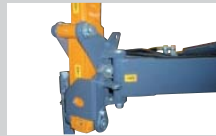
Mechanical breakaway (protection in case of obstacles).
