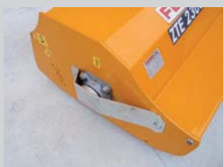
Rotor internal sealed bearings
