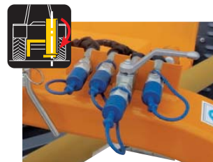
Hydraulic block tap of flail head during transport (no chains or holders).
