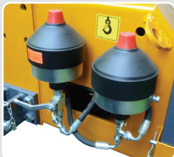
Lift float nitrogen accumulator.
