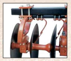
The Spring Bearing Hanger provides maximum strength without sacrificing flexibility. It also features a Wear Plate which protects the front and bottom of the Bearing Housing.
