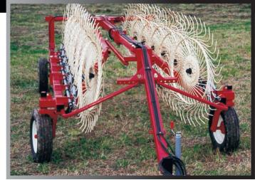
H&S Hi-Capacity rakes fold up to 8'6" or less with the touch of a lever for road transport or to go through gates.
