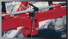
An adjustable brake band on top of the front spindle keeps the front gauge wheels from spinning in rough conditions.
