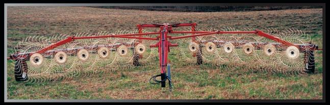
The H&S Hi-Capacity bi-fold rakes have the raking wheels positioned ahead of the rake arms, main frame beams and transport wheels. Coupled with a high and wide end of frame there are no hangup points or restrictions when raking the heaviest of hay crops.
