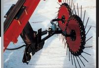
A 2 or 3 wheel center kicker assembly is optional for the Hi-Capacity rakes.
