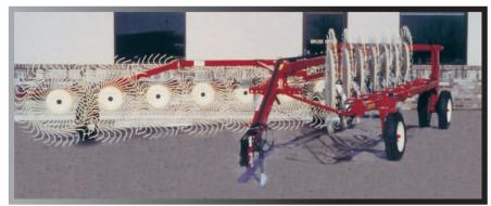
The Hi-Capacity rake can be configured as both a v-rake or with the right side open as a trailer rake.
