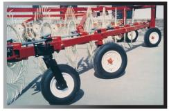
An optional set of 15" front gauge wheels for the 14 Wheel Hi-Capacity rakes help improve float over irrigation tracks or rough ground.
