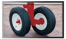
Limited oscillating offset tandem transport wheels assure a smooth, level ride, even over irrigation tracks. Standard on the 14 wheel Hi-Capacity, optional on the 12 wheel Hi-Capacity.
