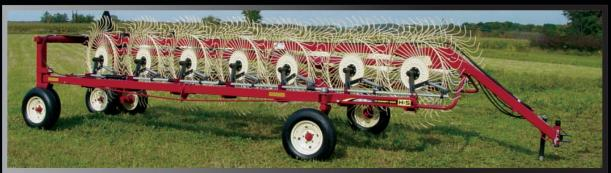
The Hi-Capacity rake opens and closes hydraulically, rake wheels are lowered and raised hydraulically, and the rake wheels float independently.
