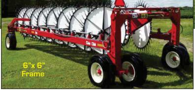
Rear Limited Oscillating Offset Tandem Axle
