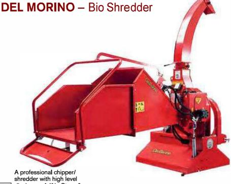
A professional chipper/ shredder with high level discharge. A "No Stress" version is available which automatically adjusts the feed rollers to prevent the engine swintching-off of the tractor. Reliability and safety are key elements of this machine.
